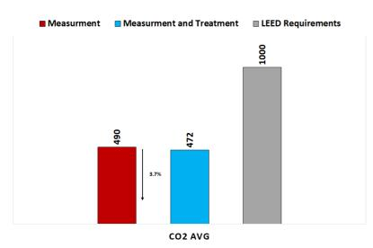
There was a slight decrease in the CO2 levels in the meeting room. Overall the CO2 level in the room is low and caused by the high flow rate of fresh air flowing into the room- something that could be more efficient and save energy if done by demand according to the AURA CO2 sensor.
