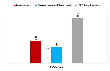
There was a significant improvement in the average value of TVOC when operating AURA with the treatment algorithm. The average TVOC decreased by 28% from 125 ppb to 90 ppb, improving the air quality of the room. Aura's Ray Filter, which has activated carbon, is responsible for the significant improvement seen.
