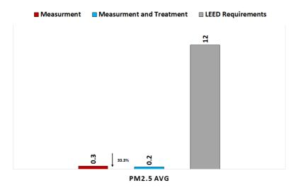
There was an improvement of 33.3% in the PM2.5 average value- that is due to the HEPA layer in the RAY filter of Aura. Overall the levels of PM2.5 are very low, much lower than the LEED requirements.
